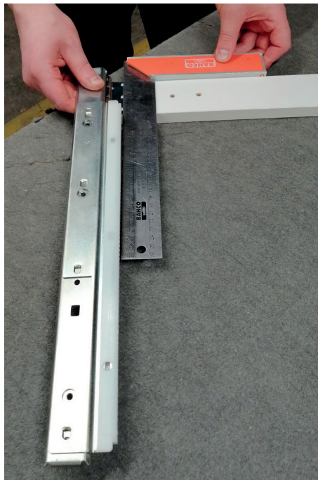
7. Ensure that the rail is at a right angle to the beam and attach the remaining screws.
