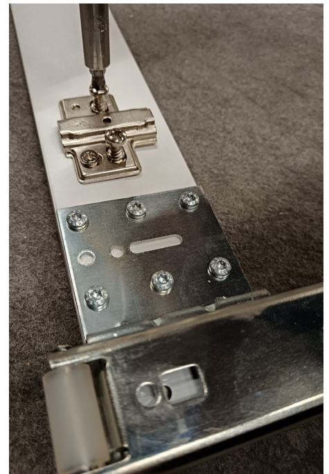
8. Install the hinge plate in place. Ensure the orientation of the hinge plate from the picture.
